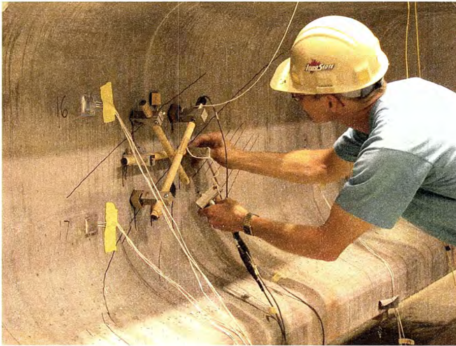
Figure 4.16. Large strain rosette gage R1 used for large-scale flexure-shear test.
