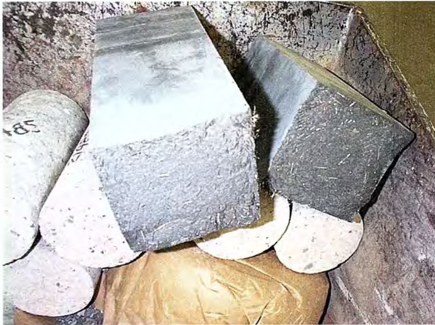
Figure 1.2. Samples of UHPC and conventional concrete.
